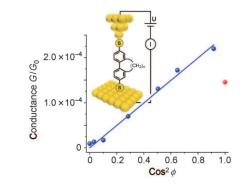
Stepwise regulation of the molecular conductance was observed in a series of eight biphenyldithiols with fixed torsion angles between the phenyl rings. These compounds were synthesized and their single-molecule conductance was investigated in an STM junction. A cos<sup>2</sup> dependence was found between the interplane torsion angle and the single-molecule conductivity (see plot).
