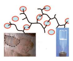
As good as new: Oil-in-water nanocontainers within an aqueous polymer network were effective for the low-impact selective cleaning of painted and gilded surfaces. Interactions with the polymer (black in the schematic illustration) did not alter the structure of the microemulsion nanodroplets (light blue and red) significantly. A photograph of an equilibrated mixture of the microemulsion and the polymer is shown.
