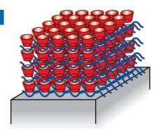
Flexible delivery vehicle: Layer-by-layer assembly and supramolecular chemistry were used to create an ultrathin-film platform technology for small-molecule delivery using a hydrolytically degradable polyion (see picture, blue waves) and a polymeric cyclodextrin (see picture, red cups).
