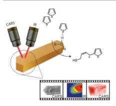
Take a look inside: The combination of coherent anti-Stokes Raman scattering and synchrotron-based IR microscopy during the catalytic conversion of thiophene derivatives on zeolite crystals yields space- and time-resolved chemically specific information without the need for labeling (see picture). The thiophene reactant is mostly present in the center of the crystal, and the product is aligned within the straight pores of the zeolites.
