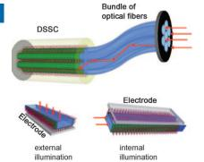
Wired up: The energy conversion efficiency of three-dimensional dye-sensitized solar cells (DSSCs) in a hybrid structure that integrates optical fibers and nanowire arrays is greater than that of a two-dimensional device. Internal axial illumination enhances the energy conversion efficiency of a rectangular fiber-based hybrid structure (see picture) by a factor of up to six compared to light illumination normal to the fiber axis from outside the device.
